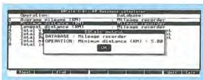
Database calculator can perform simple calculations on files created by the built-in database application.
