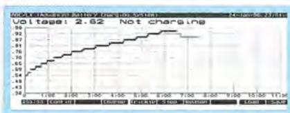
ABC/LX displays a graph showing the progress of the battery charging process.
