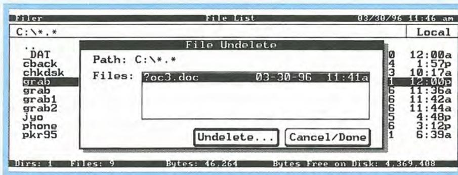
The File Undelete function displays a list of all the deleted files. Highlight the desired file and press **[ENTER]** or **[F10]** to undelete it.
