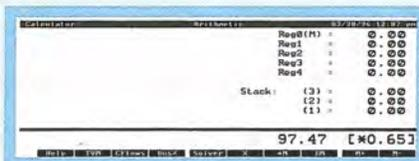
HP CALC showing constant of 0.65 in square brackets on the bottom Calc line.
